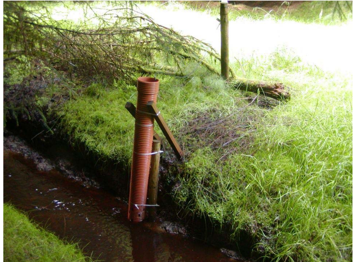
Figure 3 Water level recorder and stilling well at Flanders Moss Site 3
